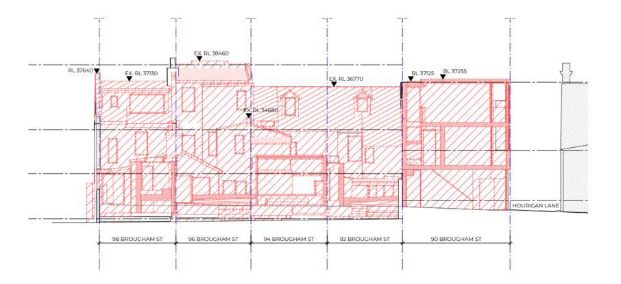
existing rear elevation (adjoining driveway) showing proposed demolition
